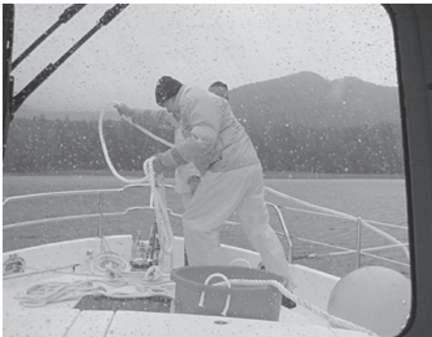
Adding a 1-inch thick back-up mooring line as storm intensifies.
